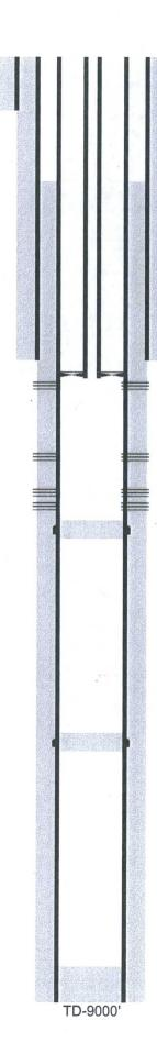
14-3/4" hole @ 451' 10-3/4" csg @ 451' w/ 470sx-TOC-Surf-Circ
