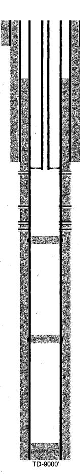
14-3/4" hole @ 451' 10-3/4" csg @ 451' w/ 470sx-TOC-Surf-Circ
