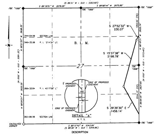
A strip of land 180 feet wide, being 3,884.99 feet or 235.454 rods in length, lying in Section 27, Township 24 South, Range 30 East, N. M. P. M., Eddy County, New Mexico, being 90 feet left and 90 feet right of the following described survey of a centerline across B. L. M. land:
