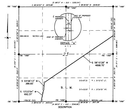
A strip of land 180 feet wide, being 5,777.72 feet or 350.165 rods in length, lying in Section 23, Township 24 South, Range 30 East, N. M. P. M., Eddy County, New Mexico, being 90 feet left and 90 feet right of the following described survey of a centerline across B. L. M. land:
