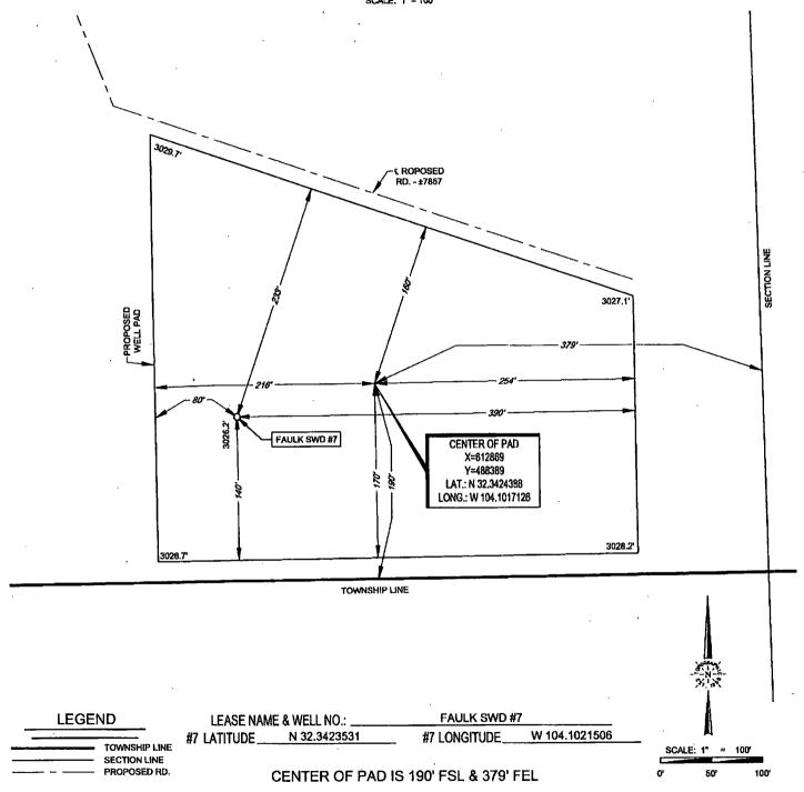
ALL BEARINGS, DISTANCES, AND COORDINATE VALUES CONTAINED HEREON ARE GRID BASED UPON THE NEW MEXICO COORDINATE SYSTEM OF 1883, EAST ZONE, U.S. SURVEY FEET
