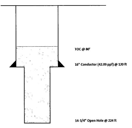
Note: Remaining 80' of conductor will be filled with cement after drilling the Height CC 6-7 Fed Com 31Y.
