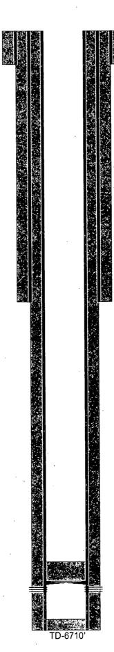
14-3/4" hole @ 374' 11-3/4" csg @ 374' w/ 320sx-TOC-Surf-Circ
