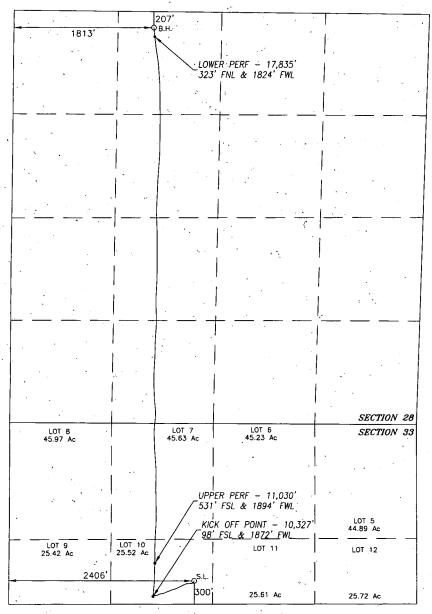
NAD 83 NME SURFACE LOCATION Y=364249.4 N X=647631.3 E LAT.=32.000938° N LONG.=103.990434° W BOREPATH SHOWN HEREON IS BASED ON DIRECTIONAL SURVEY REPORT PROVIDED BY COG OPERATING, LLC FOR THE LITTLEFIELD 33 FEDERAL COM #BOGH SUPPLIED TO HARCROW SURVEYING, LLC ON JUNE 5, 2019
