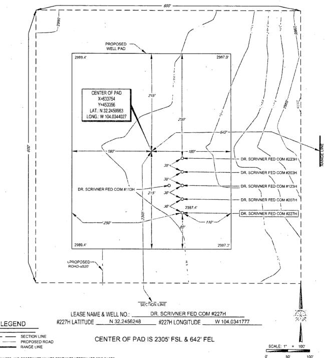
ALL BEARINGS, DISTANCES, AND COORDINATE VALUES CONTAINED HEREON ARE GRID BASED UPON THE NEW MEXICO COORDINATE SYSTEM OF 1983, EAST 20NE, U.S. SURVEY FEET
