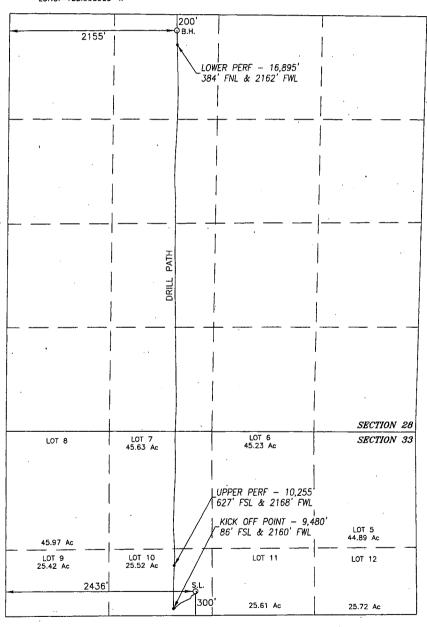
NAD 83 NME SURFACE LOCATION Y=364249.5 N X=647661.3 E LAT.=32.000938 N LONG.=103.990338' W BOREPATH SHOWN HEREON IS BASED ON DIRECTIONAL SURVEY REPORT PROVIDED BY COG OPERATING, LLC FOR THE LITTLEFIELD 33 FEDERAL COM #705H SUPPLIED TO HARCROW SURVEYING, LLC ON JUNE 5, 2019
