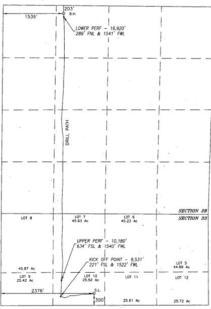
NAD 83 NME <u>SURFACE LOCATION</u> Y=364249.3 N X=647601.2 E LAT.=32.000938" N LONG.=103.990531° W BOREPATH SHOWN HEREON IS BASED ON DIRECTIONAL SURVEY REPORT PROVIDED BY COG OPERATING, LLC FOR THE LITTLEFIELD 33 FEDERAL COM #70GH SUPPLIED TO HARCROW SURVEYING, LLC ON MAY 23, 2019
