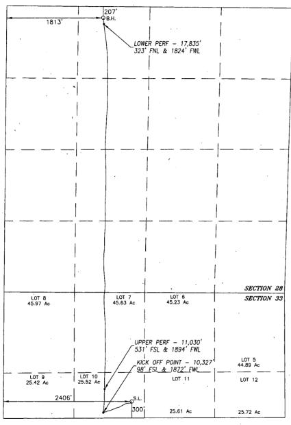
NAD 83 NME <u>SURFACE LOCATION</u> Y=364249.4 N X=647631.3 E LAT.=32.000938' N LONG.=103.990434' W BOREPATH SHOWN HEREON IS BASED ON DIRECTIONAL SURVEY REPORT PROVIDED BY COG OPERATING, LLC FOR THE LITTLEFIELD 33 FEDERAL COM #806H SUPPLIED TO HARCROW SURVEYING, LLC ON JUNE 5, 2019
