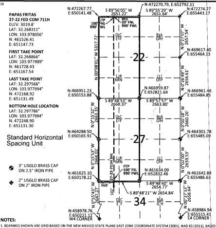
FROM GPS OBSERVATIONS, OCCUPYING A WHS CONTROL POINT (5/8" REBAR), LOCATED AT NORTH: 456034.443, EAST: 653560.641, ELEVATION: 3101.373, DETERMINED BY AN OPUS SOLUTION ON DECEMBER 3RD, 2018.
