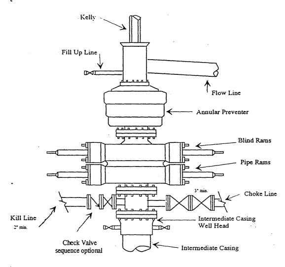
Typical 3,000 psi choke manifold assembly with at least these minimum features
