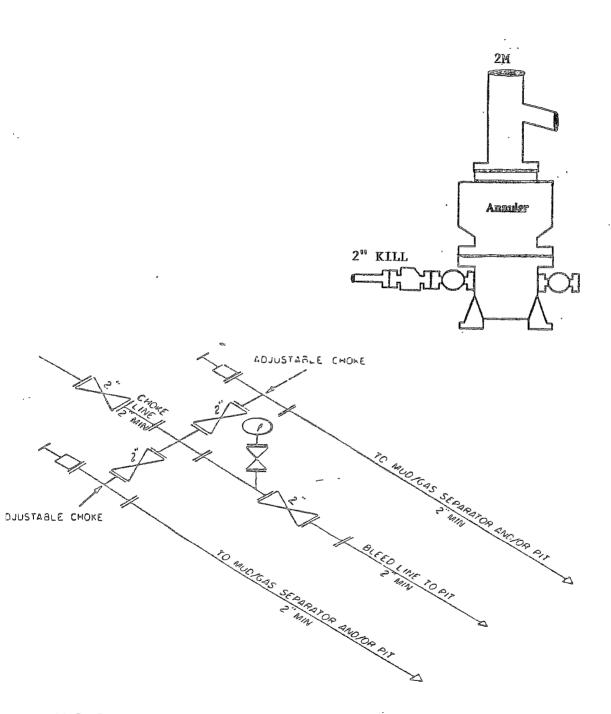
2M CHOKE MANIFOLD EQUIPMENT — CONFIGURATION OF . CHOKES
