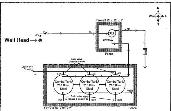
General sealing of valves and sales by tank gauging. Production phase: all drain valves (D1-D3) and sales valves (L1-L5) sealed closed. Sales phase: the tank from which sales are being made will be isolated by sealing closed the drain, fill, and any equalizer valves during sales. Draining phase: the tank being drained will be isolated by sealing closed the sales, fill, equalizer valves and drain valves on the other tanks.
