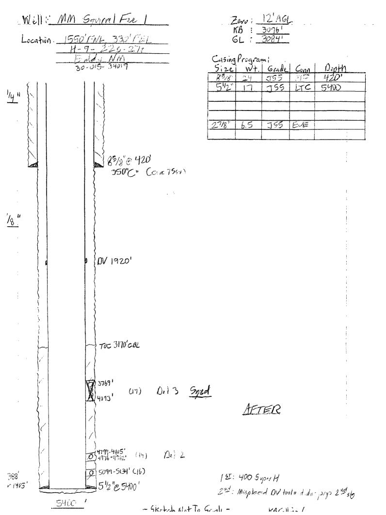
Zero: 12/16L KB: 30961 GL: 30841 Well: MM Source Fee 1 Location : 1550 FML 330 12L H-9-226 270 Casing Program: Wt. Grade Conn 755 LTC 27/81 6.5 145 EVE 85/2" @ 420 350'C" (COM 1594) 77/8" DV 1920' TOC 3170'CBL **3769'** 到4013' 0.13 (17) BEFORE O) 1771-4305' Del in 0 5097-5134' (16) - 57:63 12: 400 SuperH 5½"e5400' 17/05 1415 27 Misplaced Dy lools + 1, py 2 1date SHILL
