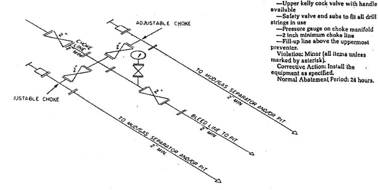
2M CHOKE MANIFOLD EQUIPMENT — CONFIGURATION OF . CHOKES
