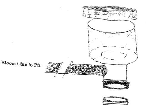
Lid Bolted onto the Wiper Rubber Chamber
