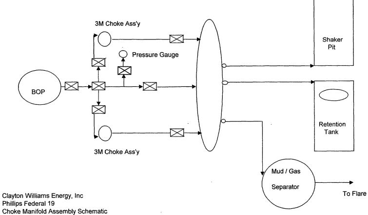
Choke Manifold Assembly Schematic Connection to Closed Looping Mud System 3M psi Rating
