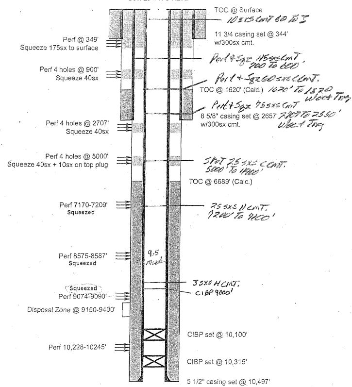
Drill out 4 squeeze jobs, drill out 3 CIBPs & squeeze 3 sets of perfs, then perforate & acidize Disposal Zone.
