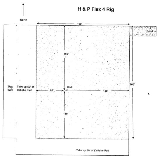
If the road comes into the Northeast corner of pad Oxy will take up and re-seed 30' on south side and 50' on west side of pad
