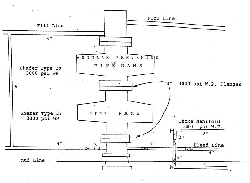
Pipe Rams are tested daily w/DP in hole; Additional tests are made after cementing casing strings.
