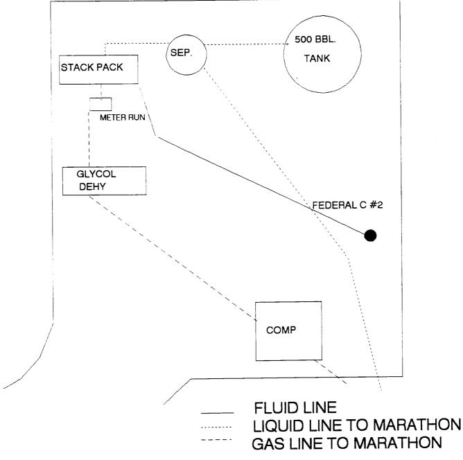
TANK IS JUST FOR SPILLS, ALL BACKPRESSURE, PRESSURE RELIEF, AND RUPTURE DISC ARE TIED INTO IT.
