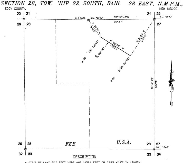
A STRIP OF LAND 50.0 FEET WIDE AND 1452.1 FEET OR 0.275 MILES IN LENGTH CROSSING U.S.A. LAND IN SECTION 28, TOWNSHIP 22 SOUTH, RANGE 28 EAST, N.M.P.M, EDDY COUNTY, NEW MEXICO, AND BEING 25.0 FEET RIGHT AND 25.0 FEET LEFT OF THE ABOVE CENTERLINE SURVEY.
