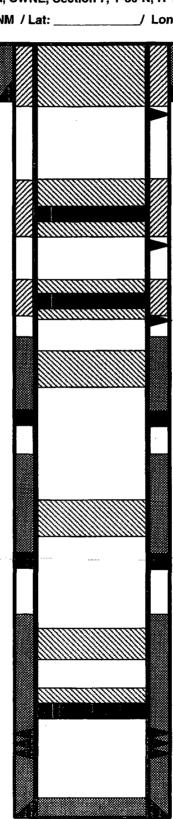
TD 6775' PBTD 6706' 9-5/8" 32.5#, Casing set @ 321' Cement with 175 sxs (Circulated to Surface)
