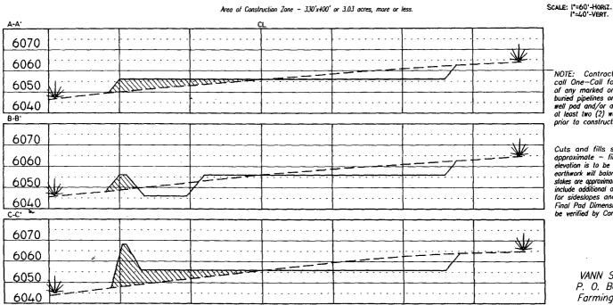
NOTE: Contractor should call One-Call for location of any marked or unmarked buried pipelines or cables on well pad and/or access road at least two (2) working days prior to construction.
