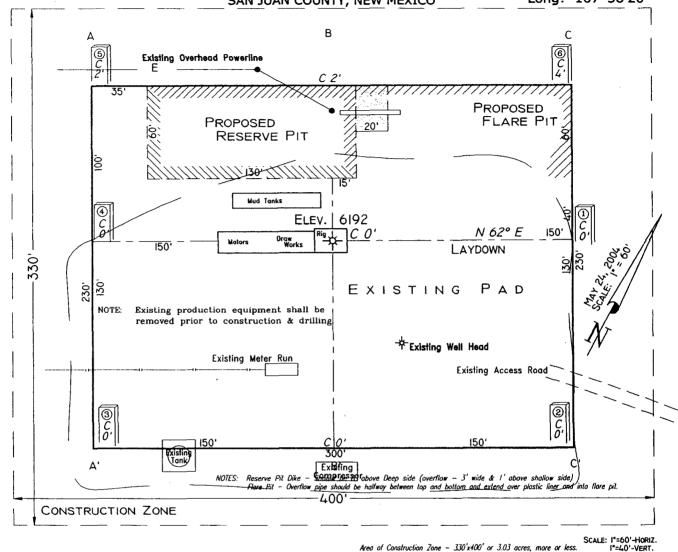
Area of Construction Zone - 330'x400' or 3.03 ocres, more or less. 6200 6190 NOTE: Contractor should 6180 6170 B-B' prior to construction. 6200 Cuts and fills shown are approximate – final finished 6190 6180 61,70 C-C, 6200 6190
