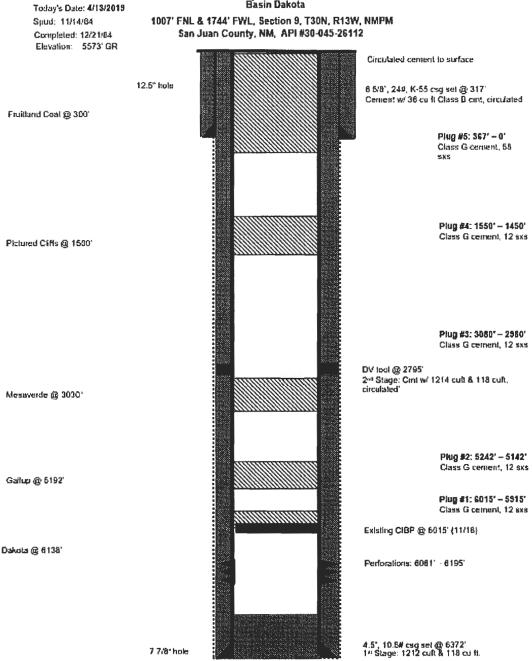
PBTD @ \$224' TD @ \$378' Hilcorp Energy P&A Final Reclamation Plan McCord #11E API: 30-045-26112 C -- Sec.09-T030N-R013W Lat: 36.83218, Long: -108.21272 Footage: 1007' FNL & 1744' FWL San Juan County, NM
