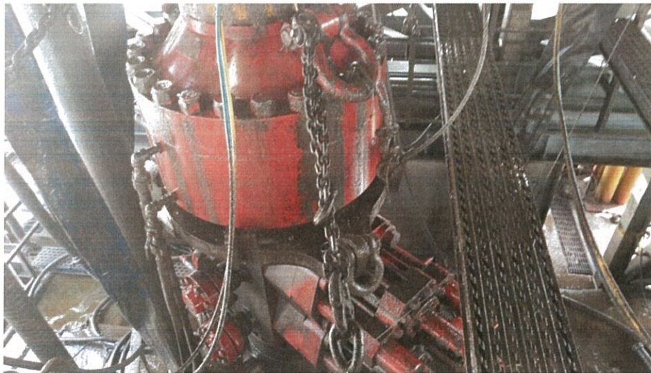
Figure 1: Winch System attached to BOP Stack
