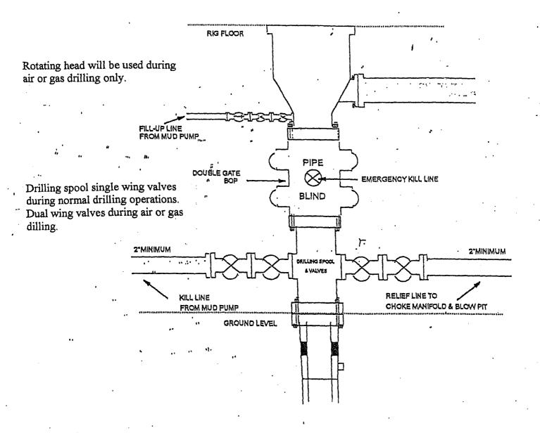
13 5/8" and 11" Bore, 2000psi minimum working pressure double gate BOP to be equipped with blind and pipe rams: A Schaffer Type 50 or equivalent rotating head to be installed on the top of the BOP. All equipment is 2000psi working pressure/ or greater.
