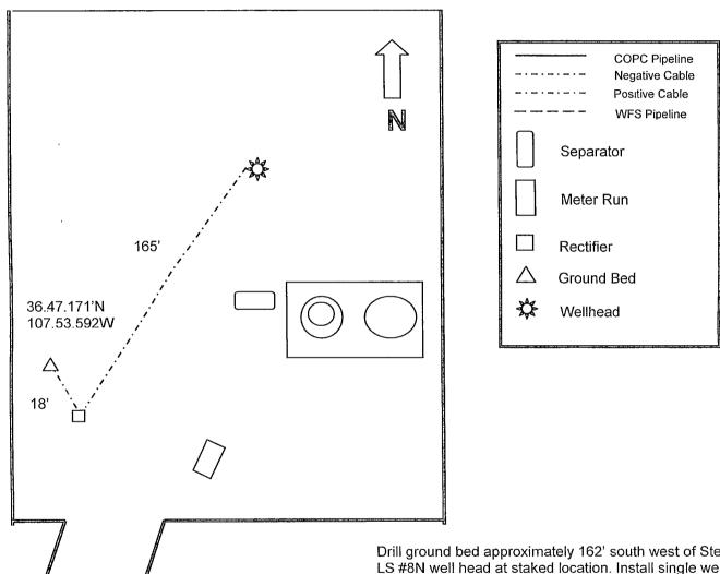
Drill ground bed approximately 162' south west of Stewart LS #8N well head at staked location. Install single well solar at staked location. Install cable to new ground bed and to Stewart LS #8N wellhead at lengths below. You may need 40' of casing and could have some boulders to drill through.
