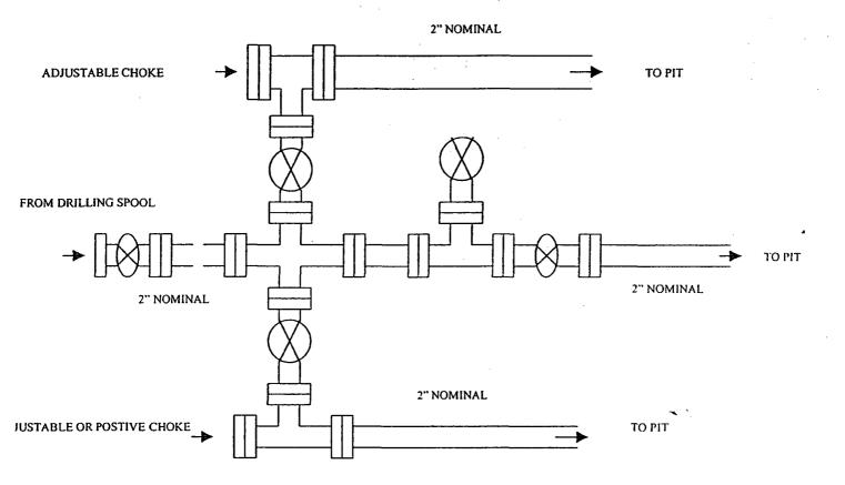
Minimum choke manifold installation from surface to Total Depth. 2" minimum, 2000 psi working pressure equipment with two chokes.
