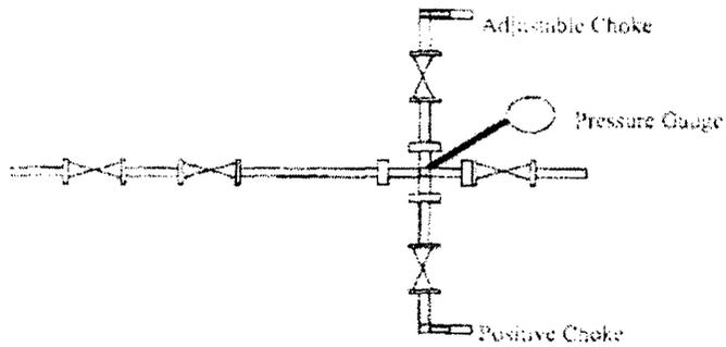
All well control equipment designed to meet or exceed the Onshore Oil and Gas Order No. 2, BLM 43 CFR 3160 requirements for 2M systems.
