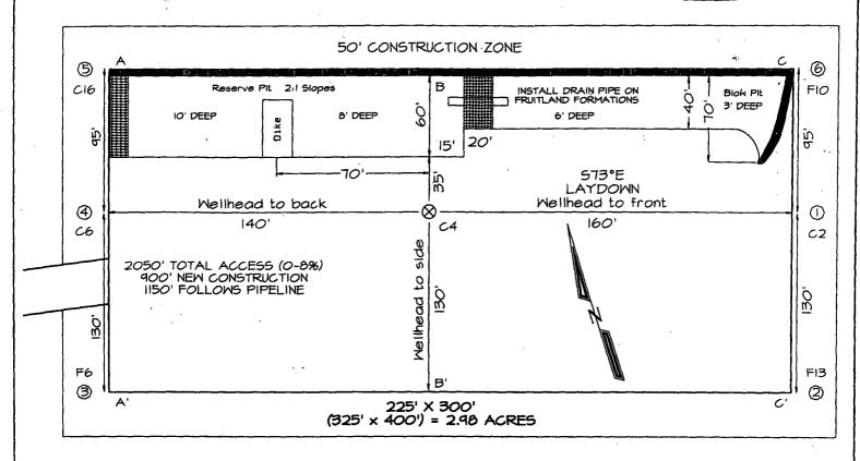
Reserve Pit Dike: to be B' above Deep side (overflow - 3' wide and 1' above shallow side). Blow Pit: overflow pipe halfway between top and bottom and to extend over plastic liner and into blow pit.
