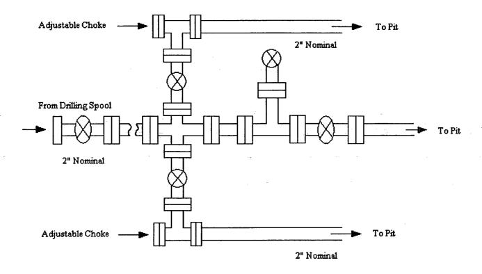
Choke manifold installed from surface to TD
