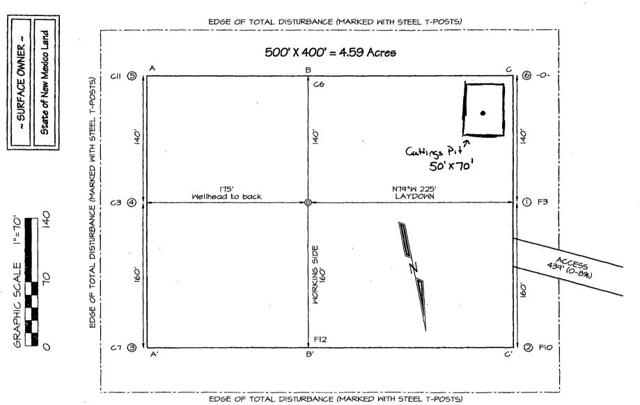
Steel T-Posts have been set to define the Edge of Disturbance limits which are 50' offset from the edge of the staked wellpad.
