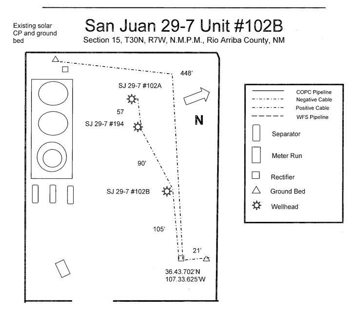
Drill ground bed approximately 123', east of #102B well head at staked location. Strip the existing duel well solar Upgrade to a multi well solar and set at staked location. Install cable to new ground bed and existing ground bed. Install Negative cable to the Solar control, San Juan 29-7 Unit #102B, #194 and #102A wellhead's at lengths below.
