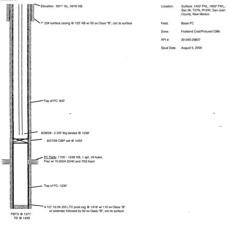
6/28/2009 -MIT. Pressured casing up to 500 psi, held for 30 minutes
