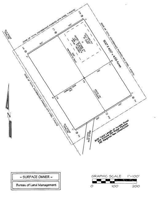
Steel T-Posts have been set to define Edge of Disturbance limits which are 50' offset from edge of staked well-pad.
