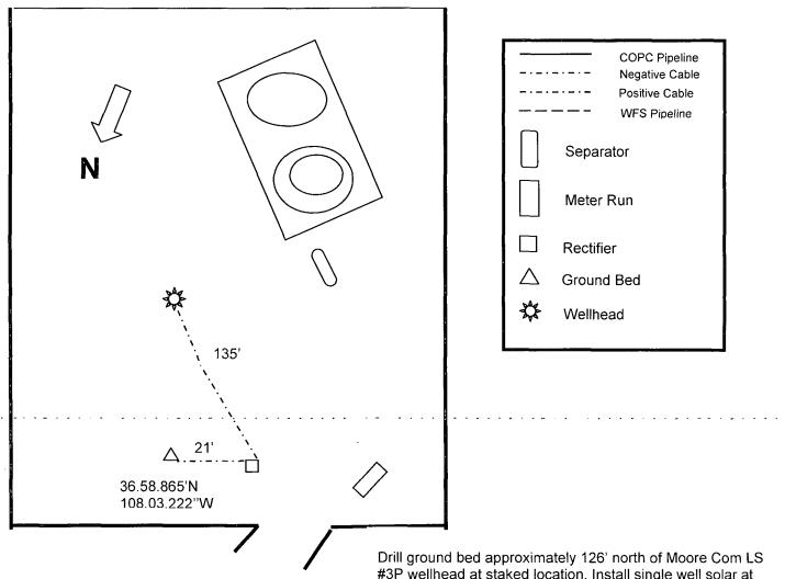
Drill ground bed approximately 126' north of Moore Com LS #3P wellhead at staked location. Install single well solar at staked location. Install cable to new ground bed and to #3P wellhead at lengths below.
