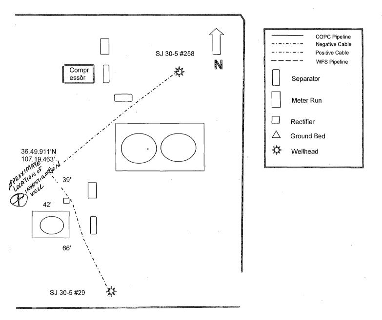
There is plenty of room to drill a test hole anywhere around the #29 well head or tank and south and west of the ground bed. We have 39' from ground bed to the rectifier, 42' from ground bed to fence, 66' from well head to corner of the fence
