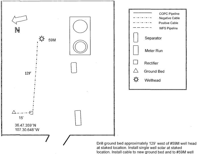
location. Install cable to new ground bed and to #5 head at lengths below.
