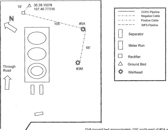
Drill ground bed approximately 105' north east of #5A well head at staked location. Install a duel well solar CP at staked location. Install cable to new ground bed and to #5A and #3M wellheads at lengths below.
