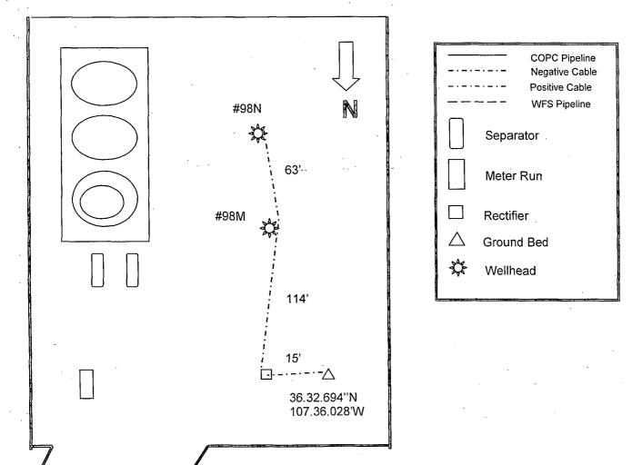
Drill ground bed approximately 120' North West of the #98M well head at staked location. Install a duel well solar CP at staked location. Install cable to new ground bed and to #98N and #98M wellheads at lengths below.
