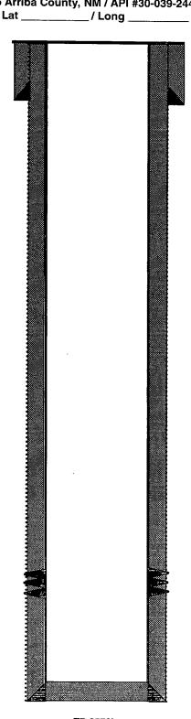
9-5/8", 36#, J-55 Casing set @ 324' Cement with 142 cuft (Circulated to Surface)
