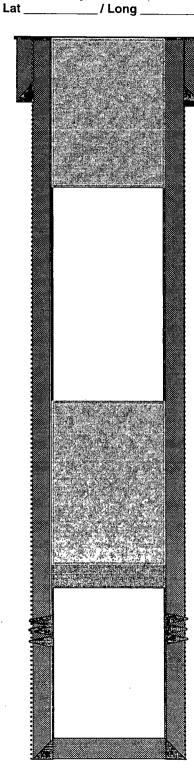
9-5/8", 36#, J-55 Casing set @ 324' Cement with 142 cuft (Circulated to Surface)
