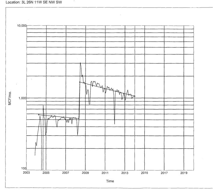
Gas Curve: Segment 1: 4/1/2004 - 5/1/2008 Start Rate: 581 mcf End Rate: 517 mcf Decline: 2.7986 Hyp Exponent: 0.000000 Goodness of Fit: 1.000000 Fit Grade: Segment 2: 5/1/2008 - 6/1/2008 Start Rate: 517 mcf End Rate: 1,659 mcf Decline: < -1000.0000 Hyp Exponent: 0.000000 Goodness of Fit: 1.000000 Fit Grade: Segment 3: 6/1/2008 - 1/1/2014 Start Rate: 1,659 mcf 1,063 mcf End Rate. Decline: 7.6635 0.000000 Hyp Exponent: 1.000000 Goodness of Fit:
