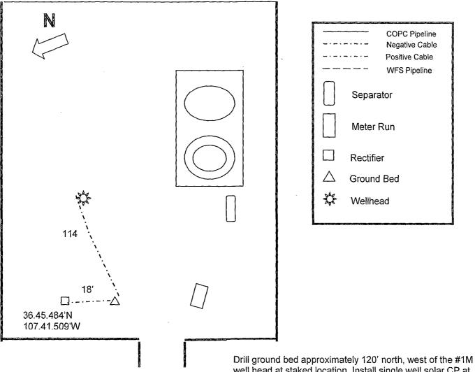
Drill ground bed approximately 120' north, west of the #1M well head at staked location. Install single well solar CP at staked location. Install cable to new ground bed and to the #1M wellheads at lengths below.
