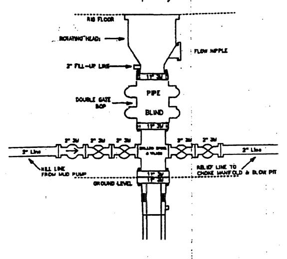
11" Bore (10" Nominal). 3000psi working pressure minimum double gate BOP to be equipped with blind and pipe rams. A rotating head on the top of the rams. All BOP equipment is 3000psi working pressure.
