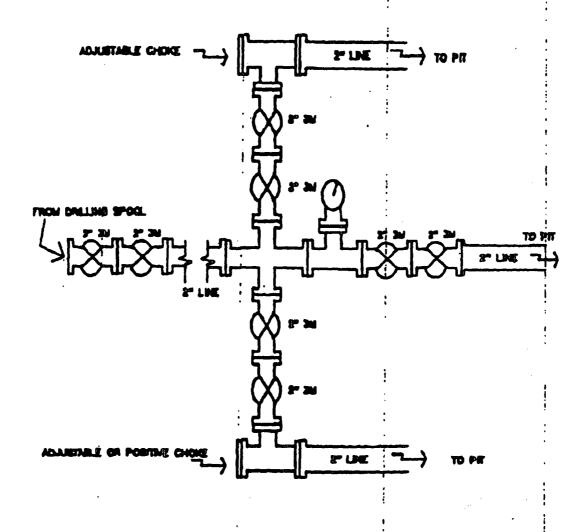
3000psi working pressure equipment with two chokes.
