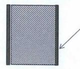
Run 13 jts, 9-5/8", 36#, K-55, LT&C, casing, set @ 302' GR. / Surface Casing -Hole Size: 12-1/4"
