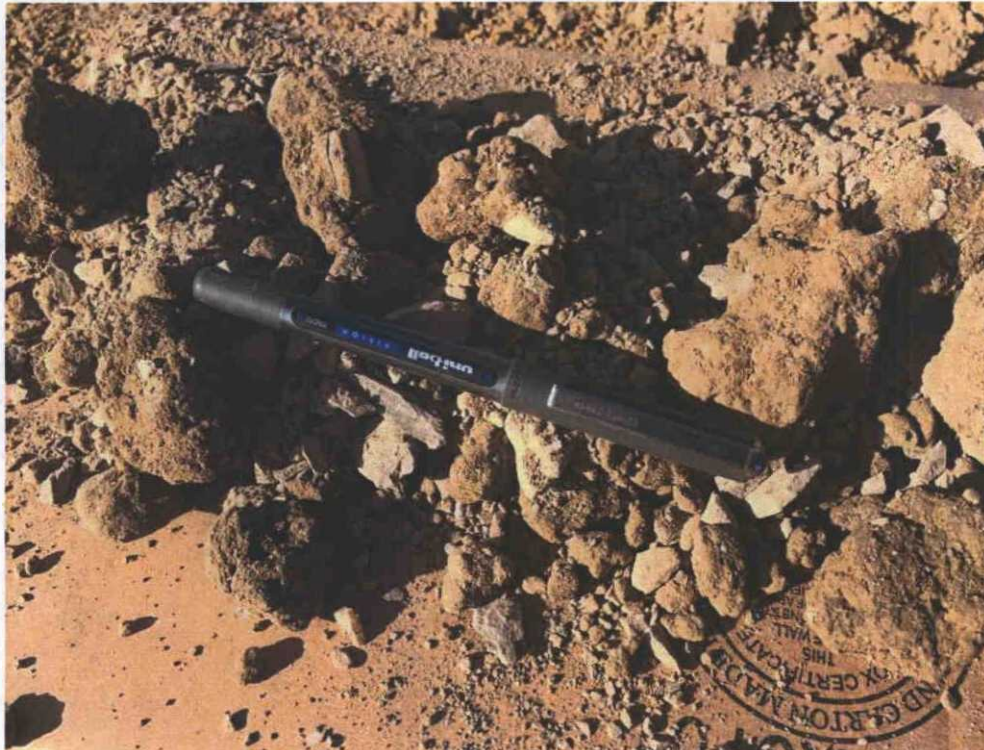
Figure 5: Mixed (3:1) drill cuttings. The soil matrix is approximately 1/3 rock, 1/3 fines, and 1/3 stabilized cuttings.
