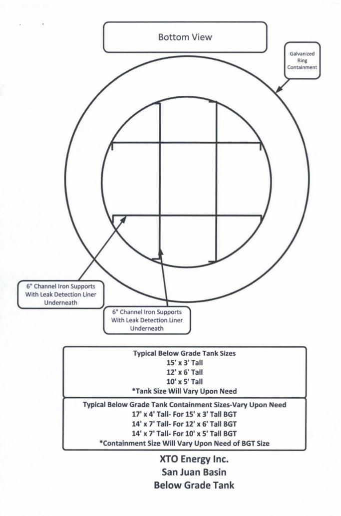
In accordance with Rule 19.15.17.11 NMAC the following information describes the general design and construction requirements of below-grade tanks on XTO Energy Inc. (XTO) locations. This is XTO's standard design and construction for all below-grade tanks. Because this below-grade tank is already installed, this design and construction plan would apply only if the below grade tank was upgraded or replaced.
